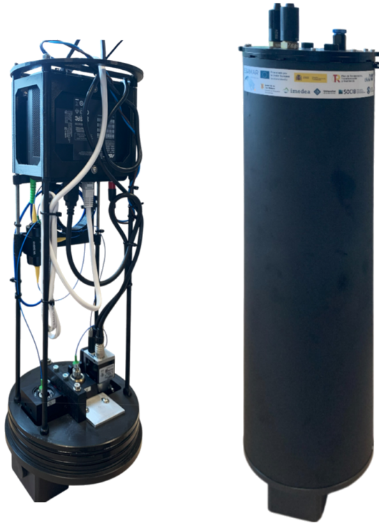
Compact DHM ® with its control unit (left) and integrated into the deployment vehicle (right).
