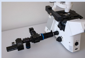
Digital Holographic Camera to be mounted on an existing fluo. microscope
