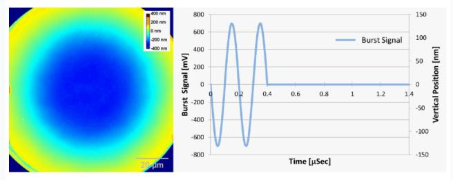
cMUT membrane response to a **burst waveform composed of two periods of a sine wave at 5 MHz** (in blue). Vertical position versus time of the membrane at three monitoring area (in red, green and yellow) randomly selected over the measurement field of view (Courtesy to Philips).
