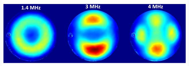
**cMUT membrane vibration amplitude map:** selection of three maps at 1.4, 3 and 4 MHz, among all those obtained by performing a DFT on each pixel of the 3D topography timesequence response.
