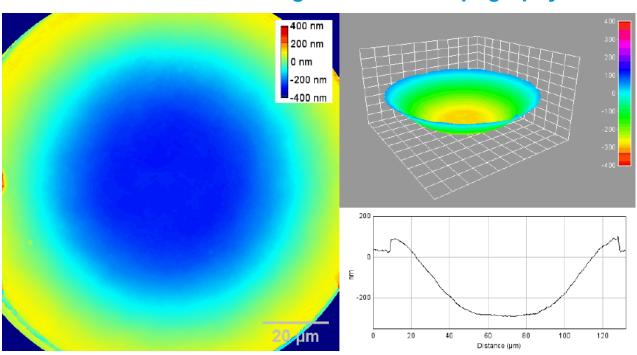
**cMUT response to a double period 5 MHz sine burst:** Left: Topography color map time-sequence animation. Upper right: 3D perspective. Bottom right: Animated profile cut. (Courtesy to Philips)
