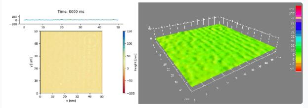
Surface-relief grating formation measured in real time with interferometric resolution at 194 fps (up to 14'000 fps in option) with a DHM® R2100.
