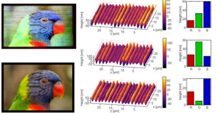
Tampere team has created periodically varying patterns on the sample surface by controlling individually two laser beams coupled into the DHM® through the optional **external optical port**.
