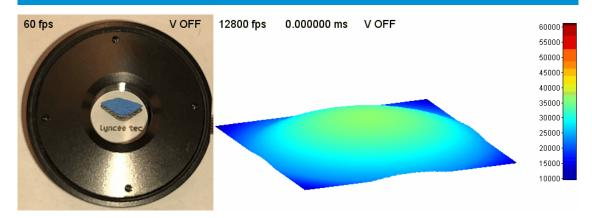
An application example is the dynamical characterization of the topography of a <u>tunable lens</u> by Optotune AG. The animation shows a comparison of the time sequence 3D topography recorded at 60 fps with normal camera and at 12'800 fps with the high speed DHM when driving the lens with a square signal at a frequency of 30Hz.
