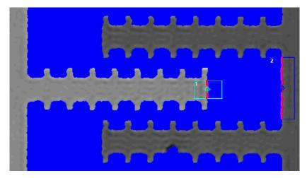
DHM® acquires information of XYZ motion for each data point in a single measurement, therefore enabling tracking of all axis simultaneously in the whole field of view.
