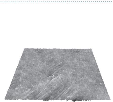
**Figure 2:** 3D representation of the roughness surface of a 1mm diameter micro-ball. The field of view is 100x100 $\mu$ m<sup>2</sup>. Measured values:  $R_a$  = 14.2nm,  $R_t$  = 270nm.
