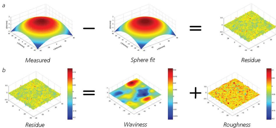
**Figure 1:** (a) Form factor removal principle: a spherical fit is subtracted to the measured surface to obtain the residual surface. (b) Roughness surface determination: the residual surface is decomposed in two parts by frequency: the waviness is composed of the low frequencies and the roughness of the high ones.
