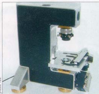
The Swiss firm Lyncée Tec has been founded to commercialize and manufacture the DHM (left). A 3D DHM image of a living mouse cortical neuron in culture (right).
