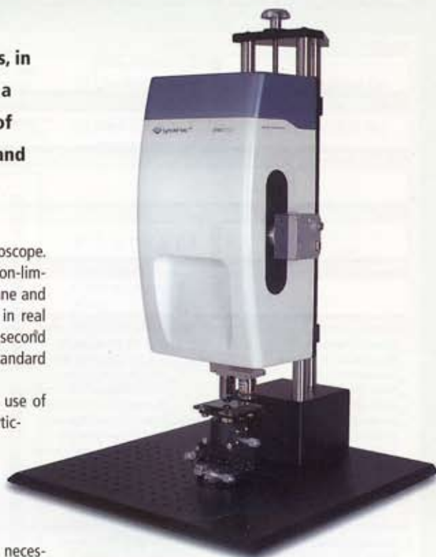
Fig. 1: DHM configured in reflection by Lyncée Tec SA. It allows 3D real time measurement at the nanometer scale of biological and material sciences samples.
